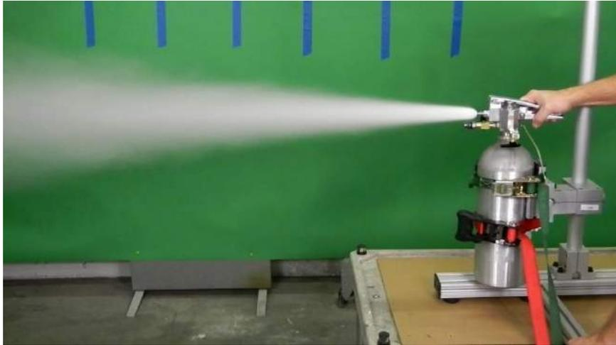
Figure 8: Discharging UHPFE on test stand
