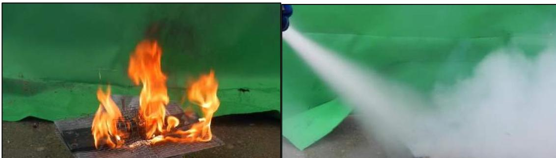
Figure 10: Battery fire (left) and UHPFE discharge (right)
