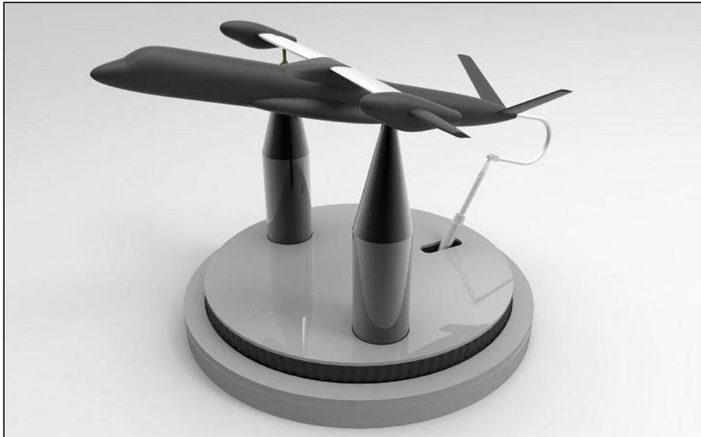
Figure 9. Rendered view of the 1/44 scale LCTR2 model on a 360 degree rotational base.
