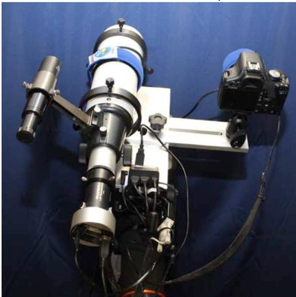
Figure 3. Research telescope. The guide-scope and camera on the left ensure accurate tracking while imaging. On the right is the modified DSLR camera used to collect the data.
