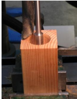
Figure 7- Drilling with the extension.
