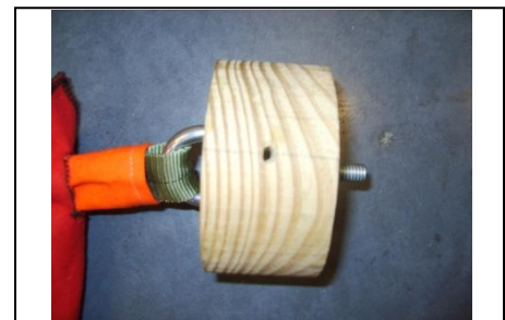
Figure 5- Upper bulkhead. The countersunk I-bolt is shown.
