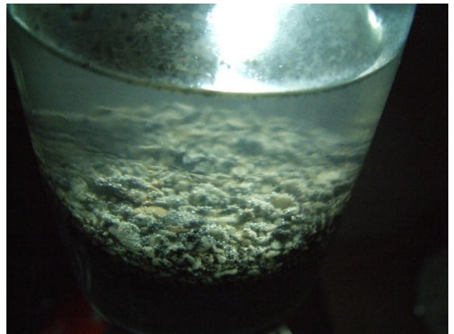
Photo 18. Restored S.C. beach sand with oxygen bubbles. Water has thin residue oil layer.
