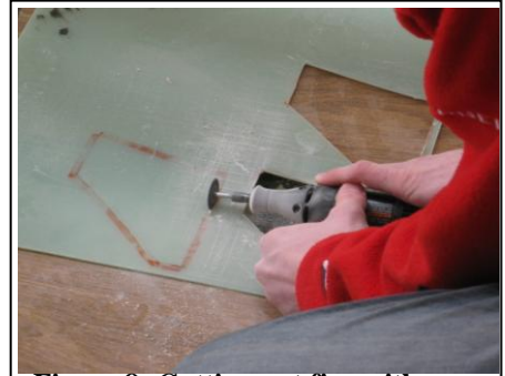
Figure 8- Cutting out fins with cutoff blade.
