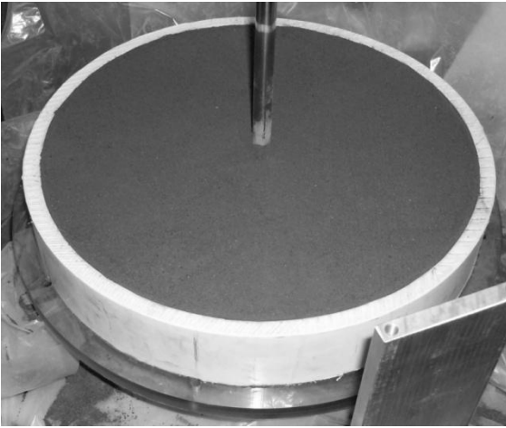
Figure 2: Filled Test Stand Before top Attached
