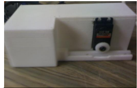
Figure 1- The breakdown voltage housing. The motor controls a gear rack to move an electrode from a gap distance of .02 cm to 1 cm.
