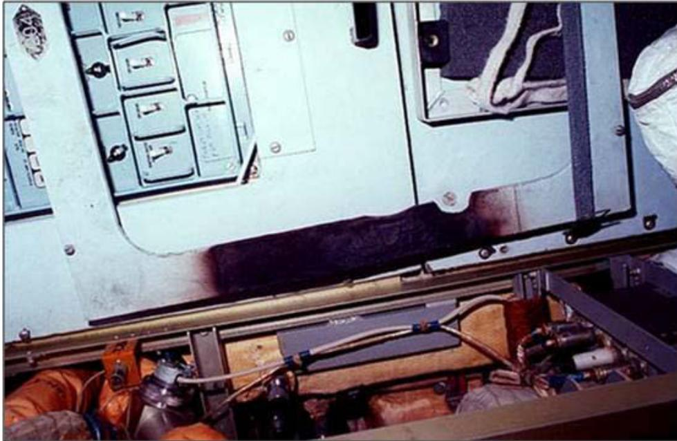
Figure 3: Fire-damaged panel onboard Mir, Credit: NASA.
