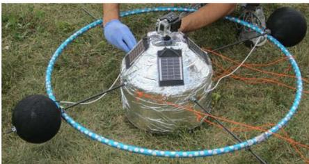
Figure 10: Final payload assembly with field probes
