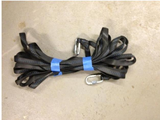
Figure 1: Shock cord and d-links used to connect the sections of the rocket
