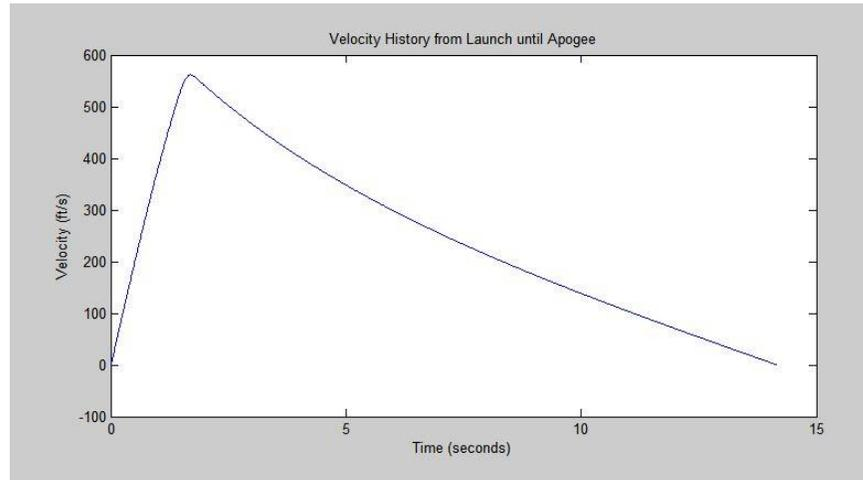
Figure 9: Velocity History Plot of the Rocket Produce by MATLAB
