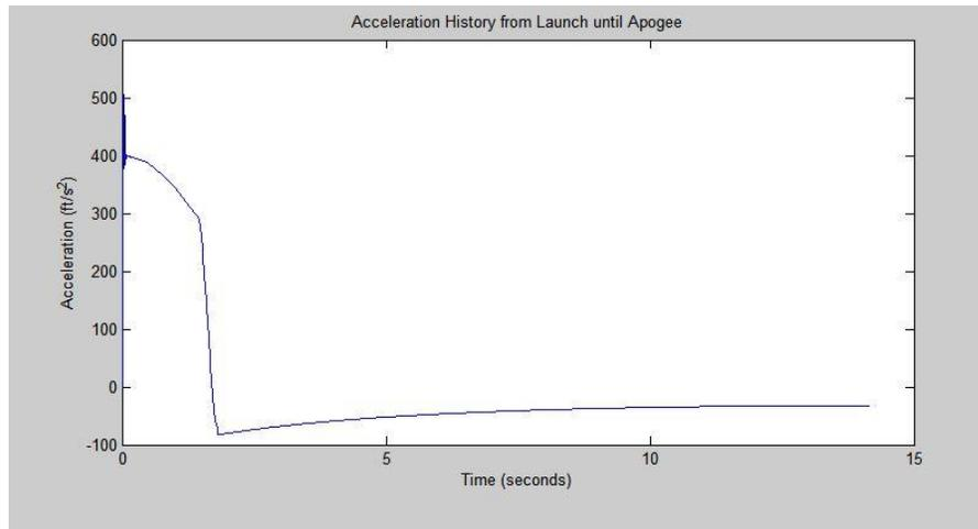
Figure 10: Acceleration History Plot of the Rocket Produce by MATLAB
