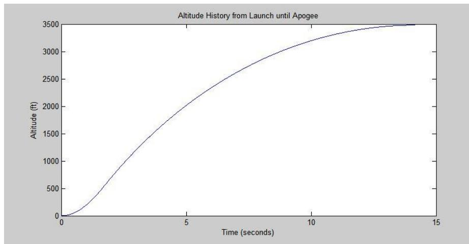
Figure 11: Anticipated Altitude Projection Plot of the Rocket Produce by MATLAB
