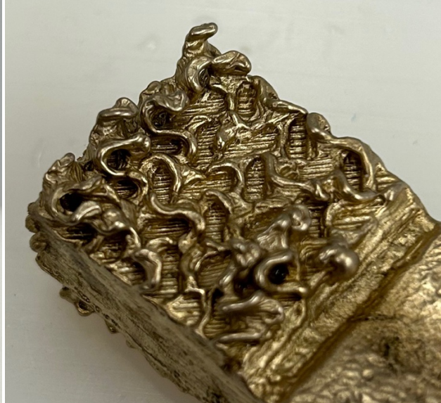
Figure 9: The first casting attempt, performed with a room temperature mold, subjected molten material to a rapid temperature change of 1015 °C. Minimal material penetration is observed in the walled cellular material cavities.
