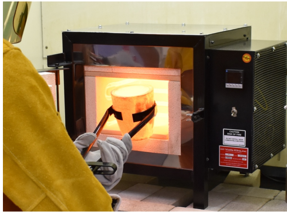
Figure 5: Immediately after removing mold from secondary oven, the mold is placed in a fume hood to minimize exposure to metal vapors and the crucible containing molten metal is removed from the furnace (left) and carefully poured into the mold (right).
