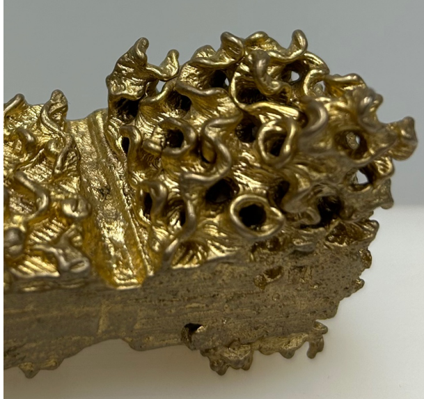
Figure 8: Using additional ventilation and a mold temperature of 275 °C, significantly improved penetration on thin features is observed; however, premature solidification continues to induce misrun defects.
