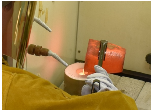
Figure 5: Immediately after removing mold from secondary oven, the mold is placed in a fume hood to minimize exposure to metal vapors and the crucible containing molten metal is removed from the furnace (left) and carefully poured into the mold (right).
