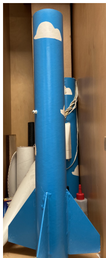
Figure 3: A post-flight image of the rocket. The upper body tube only suffered slight zippering, but the lower body tube, including each of the fins, remained intact.
