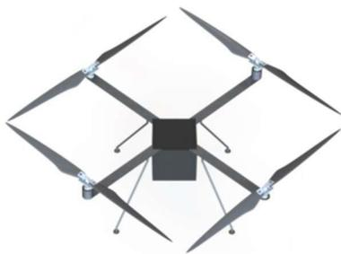
Figure 23: Overlapping Quadcopter
