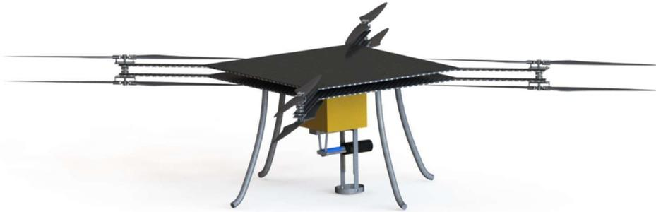
Figure 37: Drill mounted on stacked octocopter with drill in sample carrying position
