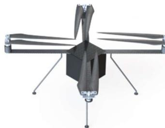
Figure 29: Folding Quadcopter
