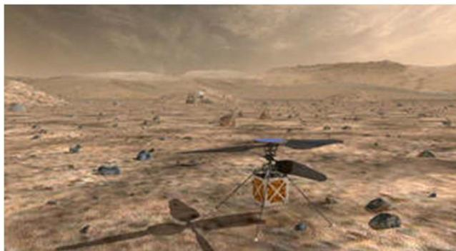
The Mars Helicopter [F2], sponsored by JPL, is part of the Mars 2020 mission as a technology demonstrator for extraterrestrial flight. The coaxial design has a rotor diameter of 1.21 meters with collective and cyclic control on both rotors and a maximum RPM of 2800. The helicopter has a
