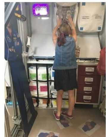
Figure 4. A 5th percentile sized female attempts to reach contents of the Emergency Medical Pack.
