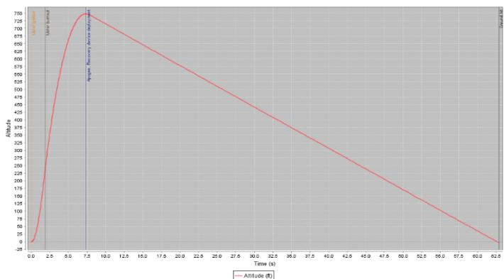
Fig. 6: Altitude vs time simulation, showing a predicted altitude of 750 ft.
