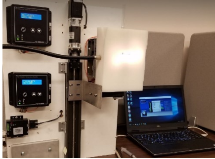
Figure 15: User Interface of ICED-T with cooler controllers and software on a laptop to control translation speed
