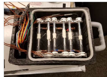
Figure 6: MMAJIC solidification tray capable of holding six quartz tubes
