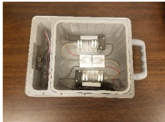
Figure 7: MMAJIC fluids tray with two syringes for fluid suspension experiments
