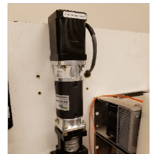
Figure 13: Stepper Motor and gearbox used for directional solidification
