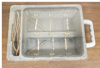
Figure 5: MMAJIC soldering tray capable of holding six soldering tests
