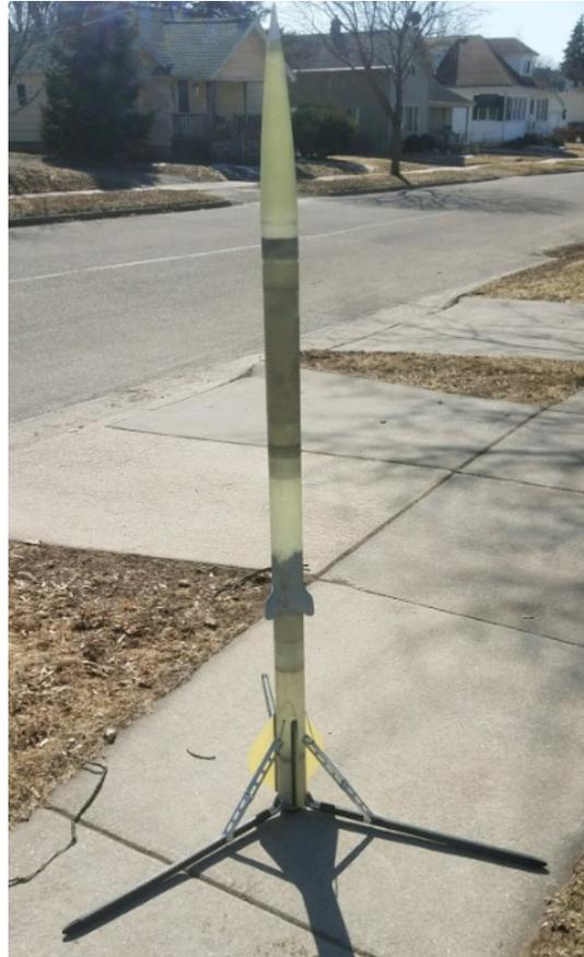
*Figure 6: Final rocket design with landing gear legs deployed*
