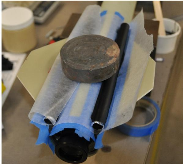
Figure 2: Fillets being applied to fins
