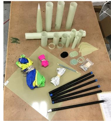
Figure 1: Parts from DX3 3" kit
