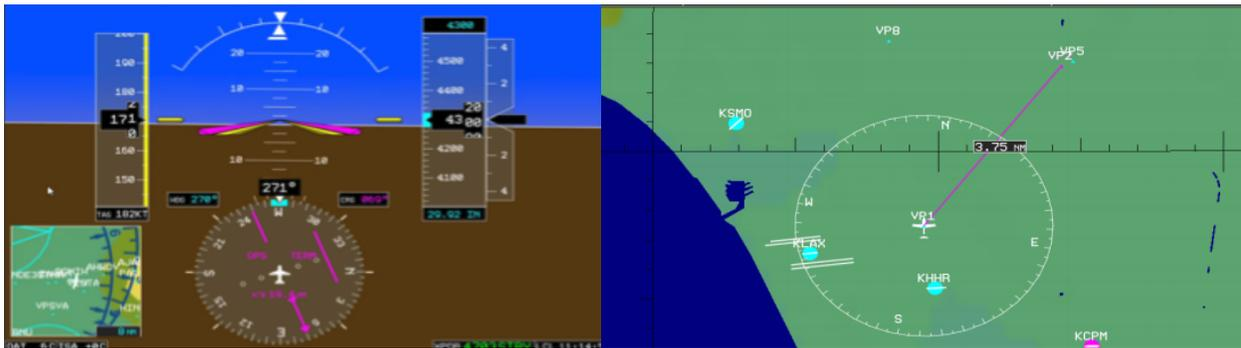
Fig. 3 (a) Primary Flight Display with Autopilot. (b) Multi-Function Display used for Navigation
