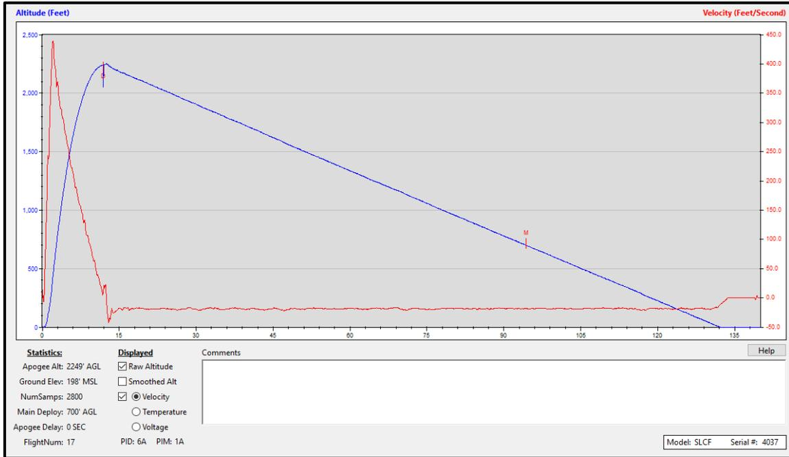
Figure 6: The Stratollogger graph of the first competition flight of Focal point. This shows the anomaly of the constant descent rate indicating main parachute deployment at apogee.
