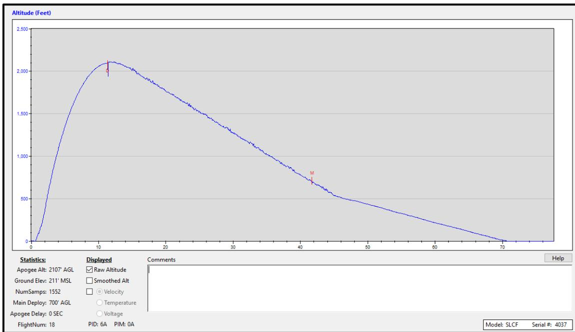
Figure 7: Stratollogger graph of the second competition flight. This was the lowest altitude of all the flights due to the camera turning sideways mid-flight, even though the effects of when the camera turned cannot directly be seen on the graph
