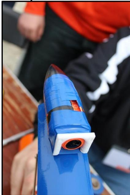
Figure 5: Improvised covering for the camera after the first flight
