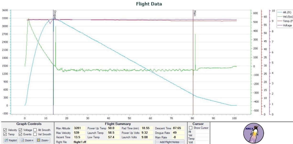
Fig. 11. Plot of altitude vs. time during the first flight. Data is from RRC3 altimeter. Picture is a screenshot taken from the program Missile Works Data Acquisition and Configuration Software by a team member.
