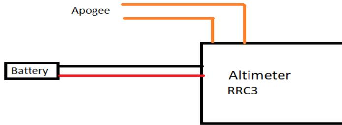
Fig. 1. A simple sketch of the components and wiring included in the electronics bay for the rocket. Sketch was created and screenshotted by team member Joseph Gawrys.
