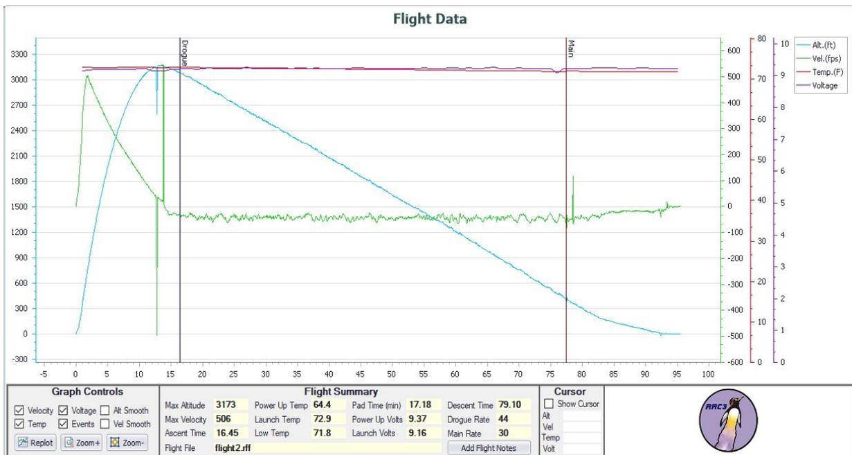
Fig. 13. Plot of altitude vs. time during the second flight. Data is from RRC3 altimeter. Picture is a screenshot taken from the program Missile Works Data Acquisition and Configuration Software by a team member.
