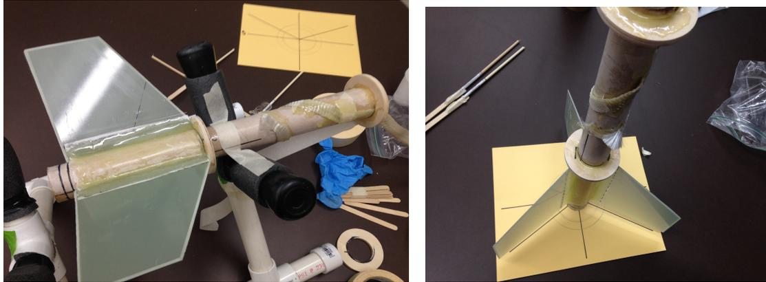
Fig. 4,5. Pictures of motor casing construction including the attachment and alignment of the fins. The fins were attached to the motor casing using epoxy. The lines on the yellow piece of paper were used to help space the fins as evenly as possible. Pictures were taken by a team member.
