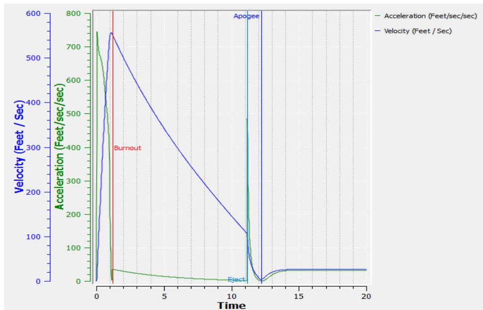
Fig. 8. Initial Rocksim Simulation with velocity and acceleration curves. Picture is a screenshot taken from Rocksim by a team member.
