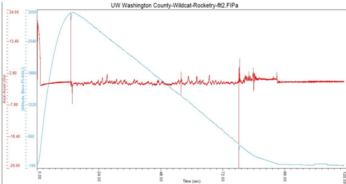
Fig. 14. Plot of Altitude vs. time during the second flight. Data is from Raven 3 altimeter. Picture is a screenshot taken from the Raven 3 data acquisition software by Dr. William Farrow of WSGC.
