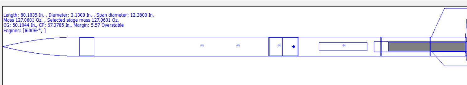
Fig. 6. A picture of the initial rocket design from Rocksim. Picture is a screenshot taken from Rocksim by a team member.
