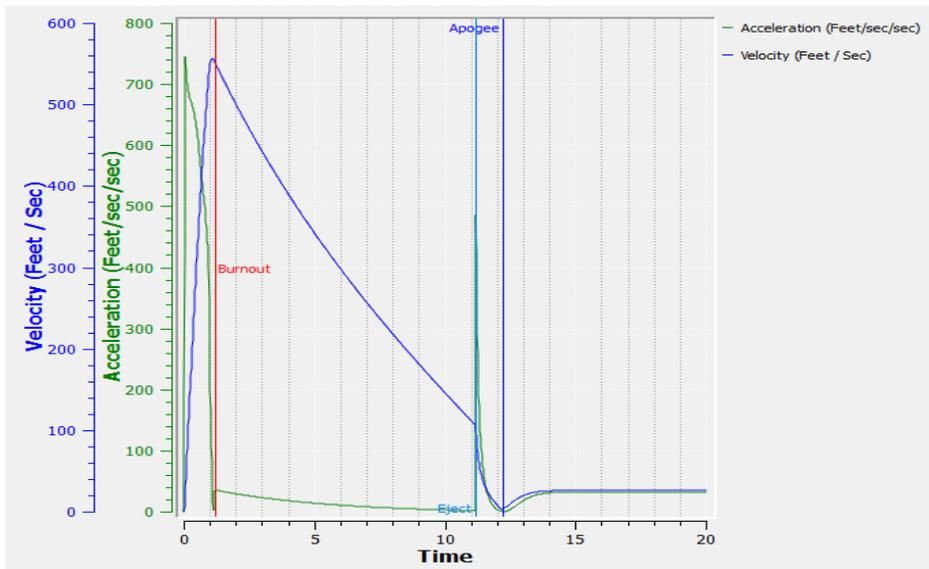
Fig. 10. An graph of predicted performance from an updated Rocksim Simulation after changes were made to the rocket design. Picture is a screenshot taken from Rocksim by a team member.
