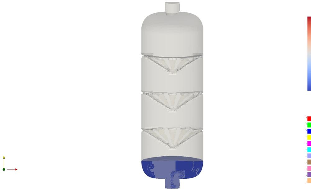
Figure 3: CFD simulations with anti-slosh baffles.
