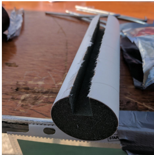
Figure 7: The C-Slot geometry of the J90 propellant grain
