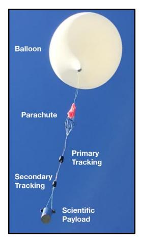
Figure 3: The balloon train as it ascended into the sky after launch
