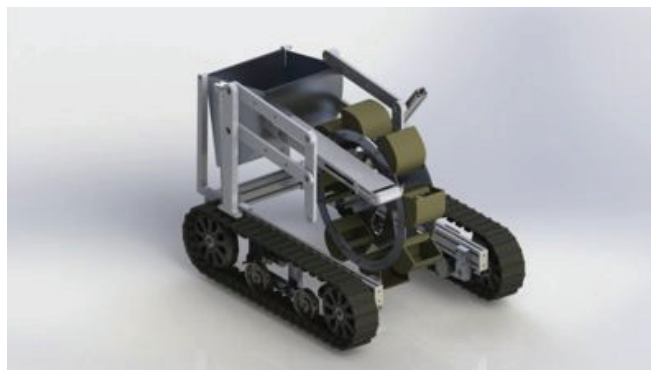
Fig. 4: BLER’s second mining system prototype used a bucket wheel
