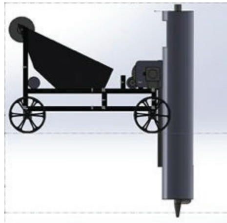
Fig. 3: BLER’s first mining system prototype used an auger
