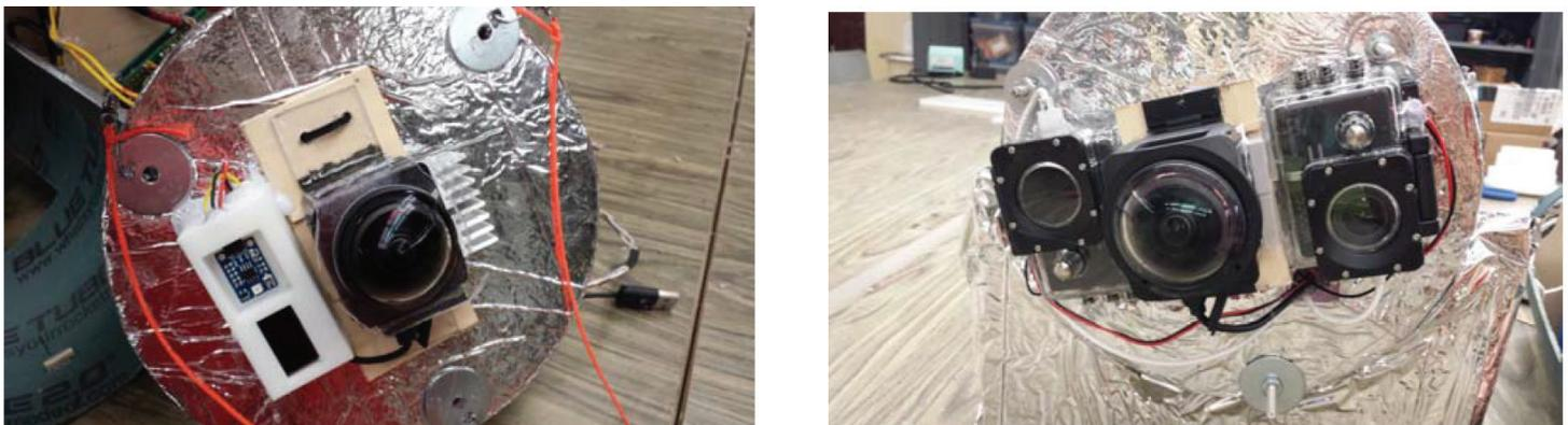
Fig 6: The left and right pictures have the top and bottom configuration respectively for the two Kodak PIXPRO SP360 4k camera. The right picture shows the 360° camera placed in between the cameras used for the infrared imaging.
