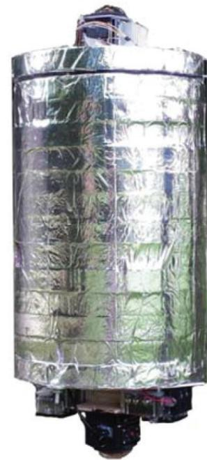
Fig 3: The outer payload shell is shown with the camera systems mounted to the top and bottom.
