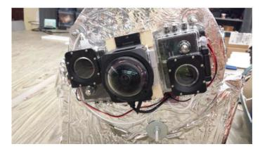
Fig 6: The left and right pictures have the top and bottom configuration respectively for the two Kodak PIXPRO SP360 4k camera. The right picture shows the 360° camera placed in between the cameras used for the infrared imaging.
