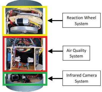
Fig 2: The interior tube and its components are shown, where each independent system mounted to a separate wood disk.
