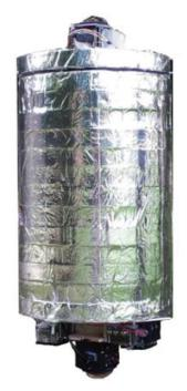
Fig 3: The outer payload shell is shown with the camera systems mounted to the top and bottom.
