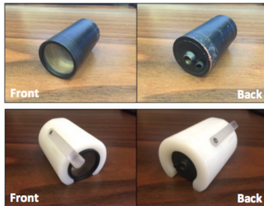
Fig. 3: Top: Camera case to be used in NBL testing. Bottom: Camera case inserted into camera mount that will be attached to the PLSS mockup for NBL testing. Design includes lever that can be depressed to allow for insertion of the camera case, but secures the case into the mount in normal position. No tools are required to insert or remove the case from the mount.
