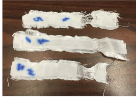
Fig. 5: 1 x 6" strips of Spectra fabric tested according to ASTM 5035 at JSC.
