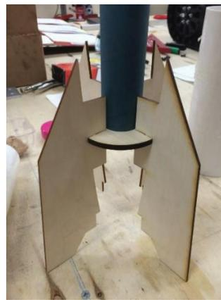
Fig. 5 and 6. Bulkhead in the middle body tube (left) and internal boat tail structure (right)
