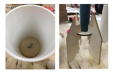
Fig. 5 and 6. Bulkhead in the middle body tube (left) and internal boat tail structure (right)
