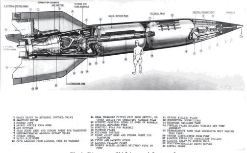
Fig 1: Diagram of V-2 internal features <sup>2</sup>
