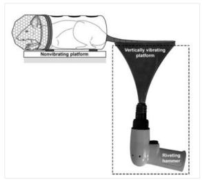
Figure 2: Vibration restraint setup. The dashed line represents the noise attenuation box that encases the riveting hammer portion of the vibration restraint (Raju etal 2011) [2].
