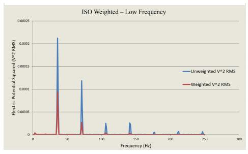
Figure 7: A magnified view detailing the lower frequencies represented in the riveting hammer signal. The y-axis scale in this plot is 320 times smaller than that of Fig. 6.
