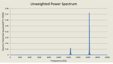
Figure 6: Although 10 frequencies were examined, the two highest at 12.4 and 16.3 kHz contain nearly all of the signal's energy. When the ISO weighting formula is applied the 16.3 kHz signal, its magnitude as well as associated risk is decreased by more than three orders of magnitude.
