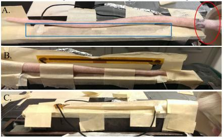
Figure 3: Step-by-step placement of the piezoelectric sensors on the vibration restraint. (A) The rat tail sits relaxed on the riveting platform. Circled in red is the fur-skin interface of the rat tail which is used to align the tail with the riveting platform. Outlined in blue is the ventral piezoelectric sensor. (B) Four tapes are placed laterally before the dorsal piezoelectric sensor is placed. (C) The dorsal piezoelectric sensor is then secured.
