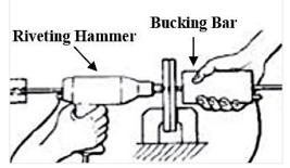
Figure 1: Demonstration of how the riveting hammer and bucking bar are used in unison to set a rivet. (Dandanell and Engstrom, 1986) [1]
