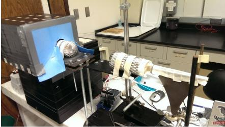
Figure 4: Loaded vibration restraint (left) and loaded control restraint (right). The NI hardware sits beneath the suspended restraints.
