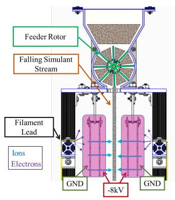
Figure 3. Operation of the SWIM device. The anode and cathode grids are ~1.6 cm apart. Each grid is ~18 cm by 10 cm by 0.3 cm thick. Each grid is approximately 90% open with 2.5 cm width gap openings.
