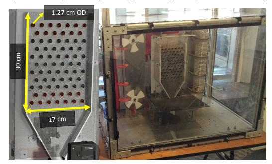
Figure 6. Pipe matrix cross section (left) and partially constructed GFX iteration 2 (right) at the 2015 Engineering Expo
