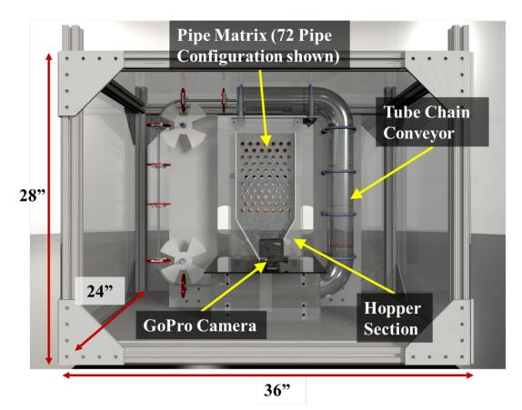
Figure 5. Updated GFX design illustrating the new pipe matrix/hopper design and tube chain conveyor.
