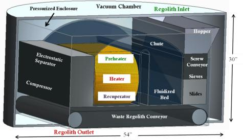
Figure 1. Concept of the HEAT system with a heat pipe heat exchanger shown in gold color
