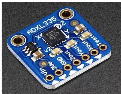
Figure 3: Three-axis Accelerometer
