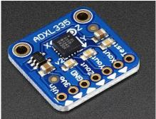
Figure 3: Three-axis Accelerometer
