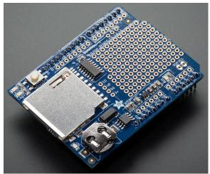
Figure 4: Adafruit 1141 SD shield for the Arduino Uno
